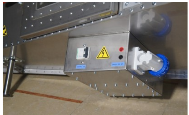
Line filters box
